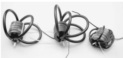
Figure 20.26 – Typical transmitting wound-coax common-mode chokes suitable for use on HF ham bands.
