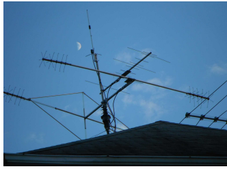
Mini Quad on roof with 2 meter/440 Yagi and Cushcraft Dual Band Ringo stacked above.
